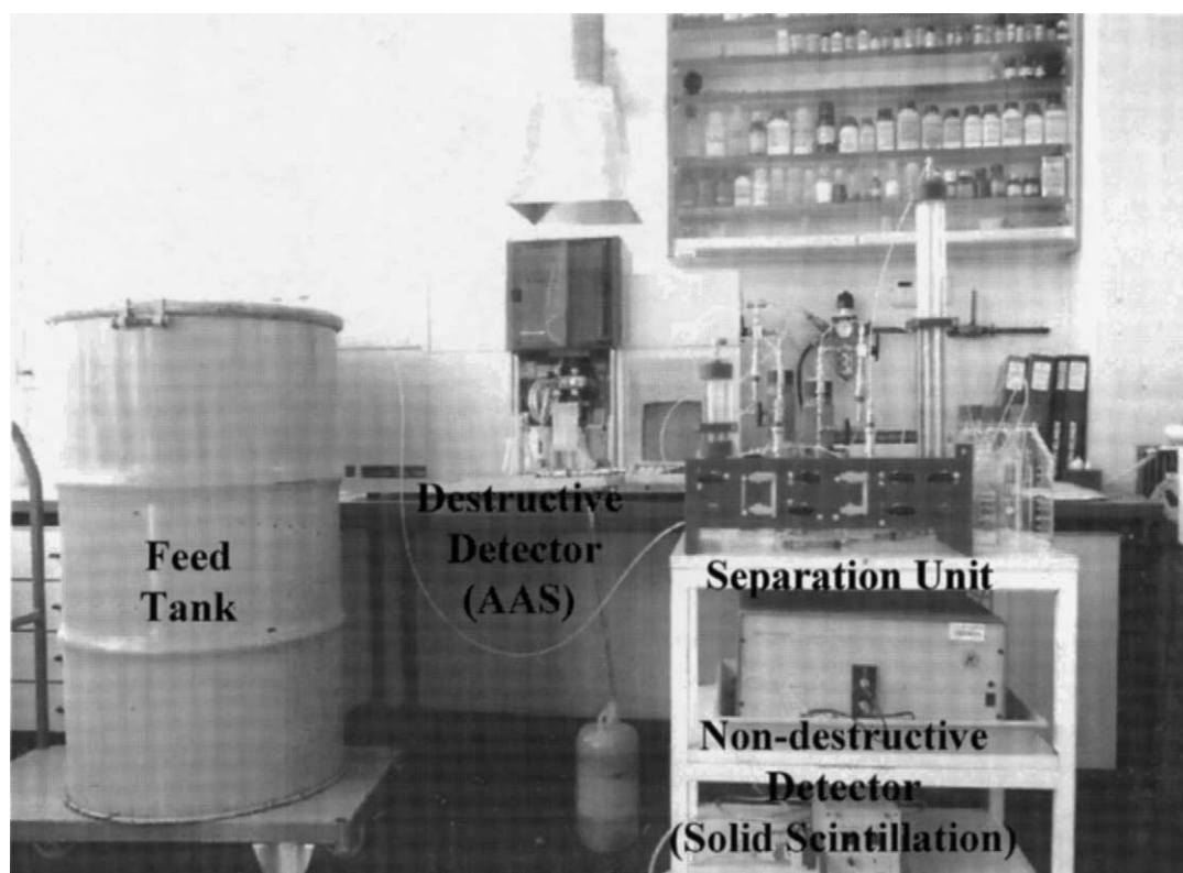
Fig. 4. Separation unit with monitor (atomic absorption spectrometer) and 200L supply tank.
